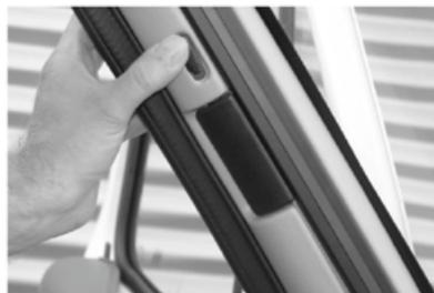
Lock front system by pulling down slider (on both sides).
